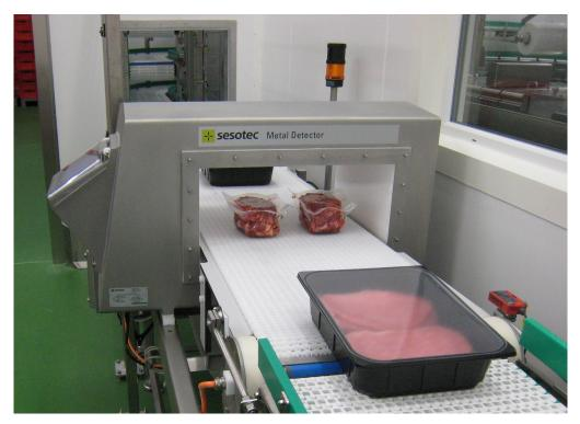
The metal detector INTUITY with multi-simultaneous-frequency technology in the inspection of very different products.
