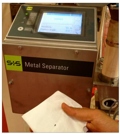
For Al-Yemeni Cafe the RAPID 8000's high sensitivity to all types of metal was the deciding factor. Even small contaminants, as shown in the picture, are easily detected.
