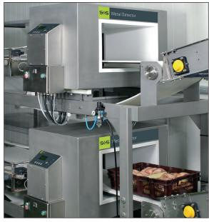
Installation example: GLS metal detectors installed in two production lines to analyse poultry. (old version)
